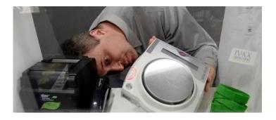
**During the scale inspection**, the inspector may find that your scale is inaccurate and/or fails to meet other technical standards. Depending on the problem, the inspector will inform you of the necessary corrective actions or the scale may be rejected/tagged "out of order." If your scale is rejected, you will have to contact a service agency registered with CDFA DMS to have the device repaired and corrected before you are able to use the scale again.
